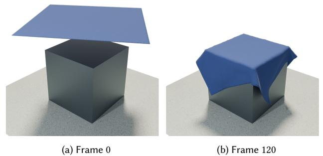
Fig. 8. Sharp Corner: stable simulation of cloth mesh on sharp corner obstacle, with rich and non-smooth contacts.
