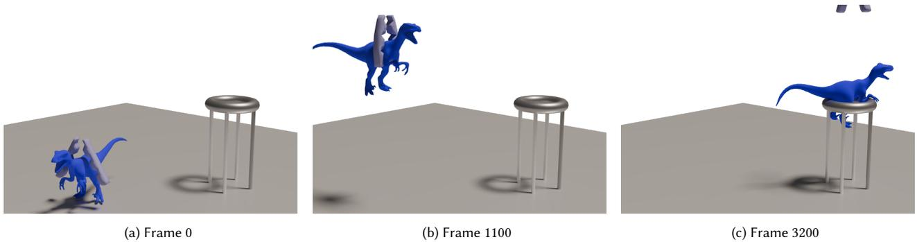
Fig. 2. Grabbing Raptor: stable catching of an elastic raptor with a soft gripper actuated by cables. Lifting, rotating, and moving the raptor by the fingers are complex operations where friction constraints are necessary. Gripper details can be seen at Appendix.C.
