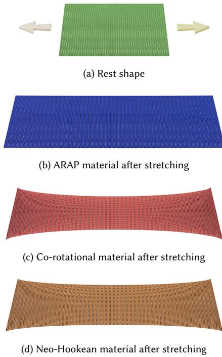
Fig. 6. Cloth Extension: capability of volume preservation with different elastic materials.
