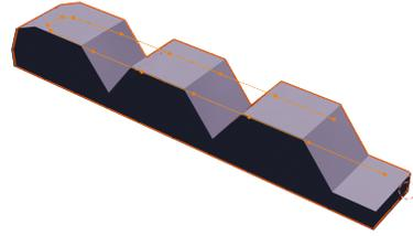
Fig. 11. Soft gripper driven by cables (simulated with bilateral constraints, highlighted with orange lines).
