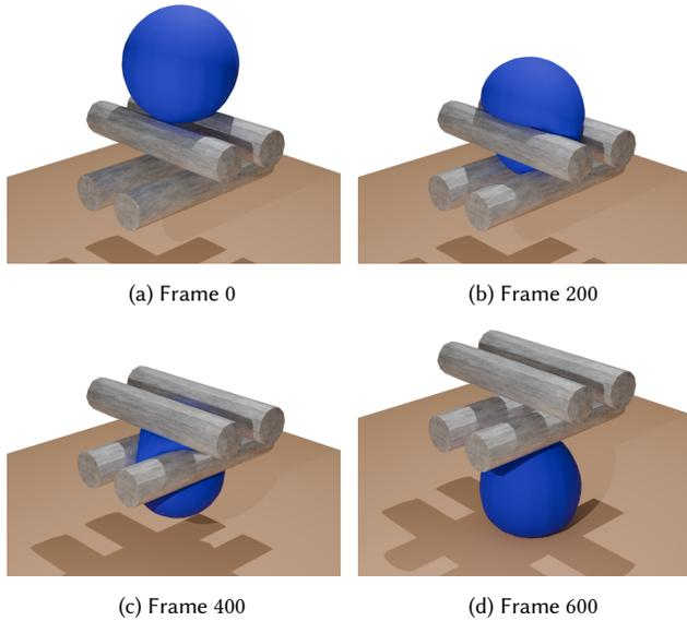
Fig. 9. Squeezing Ball: the rolling cylinders strongly squeeze the soft ball, thereby generating large frictional forces (with  $\mu = 0.5$ ) that drive the ball through the gaps.
