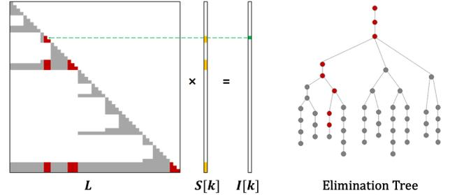
Fig. 3. Sparse solution: after reducing the matrix pattern fill-in through nested dissection, the Cholesky factor  $\mathbf{L}$  is reordered and partitioned into sub-blocks. For a given column  $k$  in the identity matrix  $\mathbf{I}$ , the requisite structure to be processed in  $\mathbf{L}$  consists of  $k$  and its ancestors (red nodes) in the elimination tree.
