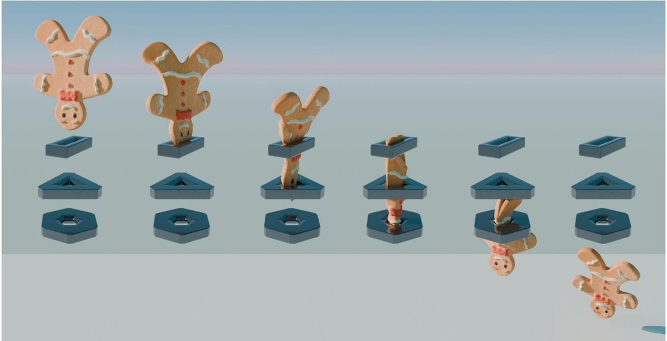
Fig. 1. Crossing Gingerbread Man: we propose a new framework for stable simulation of hyperelastic materials with nodes under large deformation and generic contact constraints in real-time. Pulling the gingerbread man (58.5k DoFs for a single object) through the thin and irregular obstacles is simulated at 11.95ms/iteration using 5 local-global iterations per frame when maximum contact pairs are involved (800 contact constraints).
